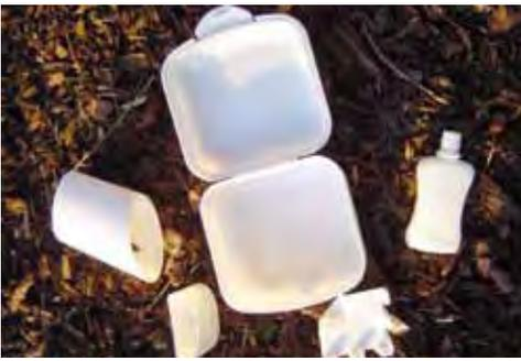
Containers made of Arboblend® containing cellulose (Source: Tecnar)
