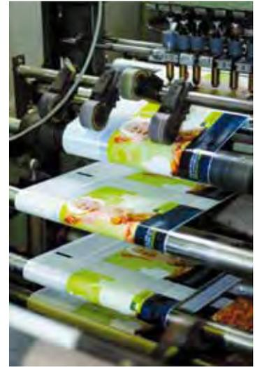
Processing foils made of bioplastics (Source: alesco)
